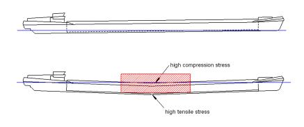
strength of the bottom steel plates, the vessel folds in the middle.
