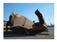
After salvage of the wreck, the typical failure mechanism as described above could be clearly noted; the barges' bottom was bent downwards in transverse direction, its sides were pushed inwards and its hatch coaming was heavily buckled.
