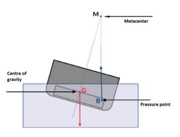
After the metacenter height (distance G-M) of a ship is determined for a particular load condition, it may need to be adjusted as a result of the presence of free liquid surfaces. These are due to the fact that tanks are not completely filled or because there is water on the load (think of loading sand barge vessels at dredgers).
